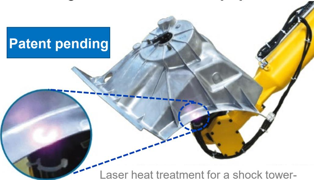
Laser heat treatment for a shock tower-shaped product
